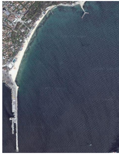
Figure 4-1 Varna beach with the breakwater (south) and Y-groyne (north).
