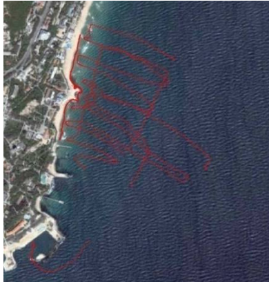
Figure 3-4 Path that has been sailed to measure the bathymetry
