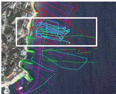
Figure 3-5 Paths that have been sailed for measuring the bathymetry over different years, including area of interest enclosed in the white rectangle
