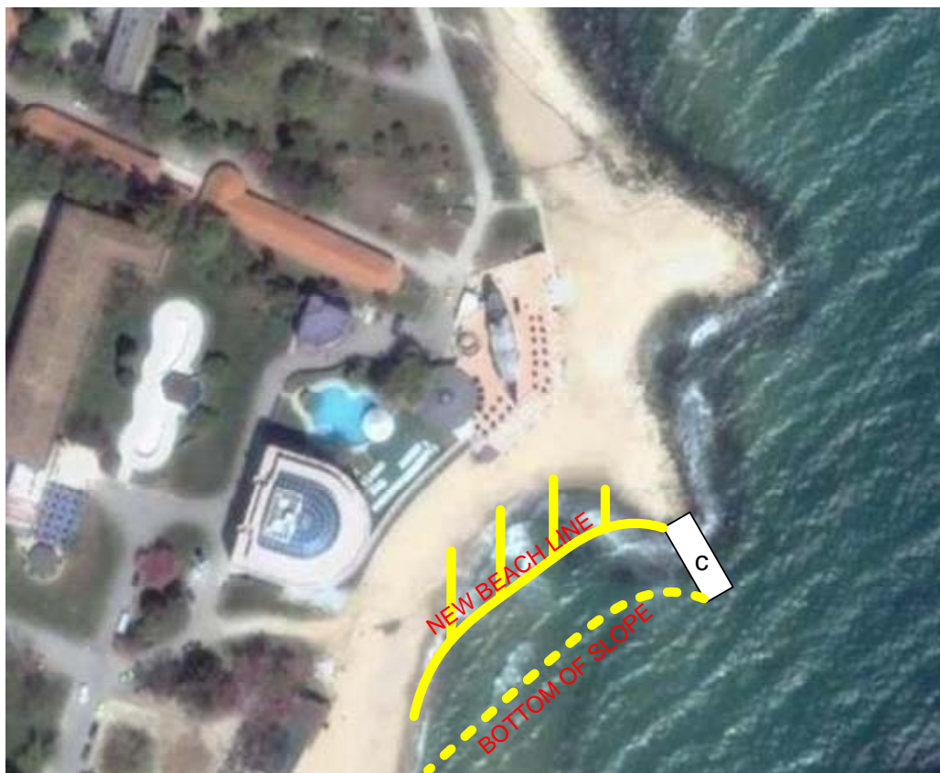
Figure 9-4 – Impact of extended groyne on coastline and beach width
