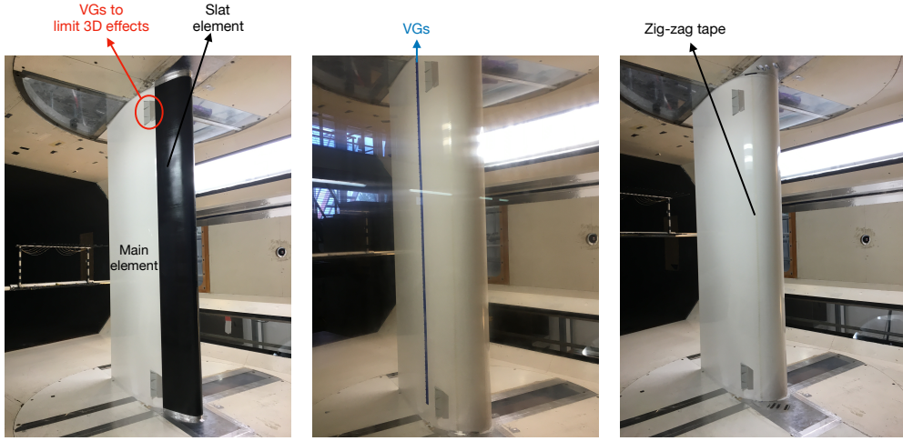
Figure 3: Photos of the experimental setup: main profile with slat element (left), main profile with vortex generators (centre), main profile with zig-zag tape (right).
