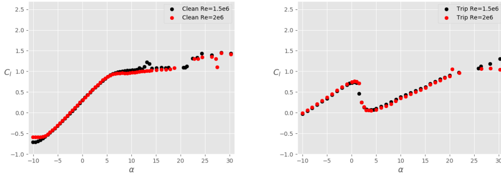
Figure 17: Lift coefficient C_l as a function of the angle of attack \alpha for the main airfoil (without slat) at two Reynolds numbers: Re = 1.5 \cdot 10^6 (black) and Re = 2 \cdot 10^6 (red). Left: clean airfoil; right: trip airfoil.
