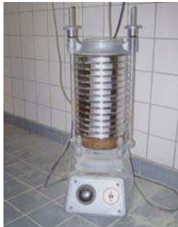
Figure 5 Drying of the sediment, stack of sieves and sieve machine
