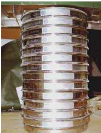
Figure 5 Drying of the sediment, stack of sieves and sieve machine
