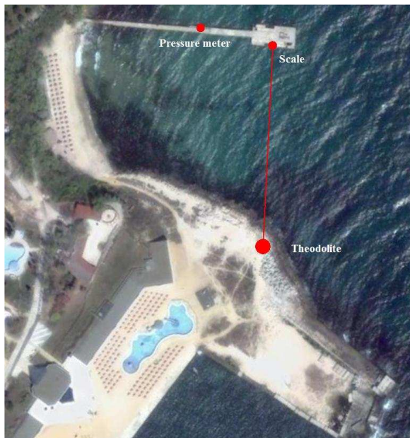
Figure 22 Position of the pressure meter, scale, and theodolite
