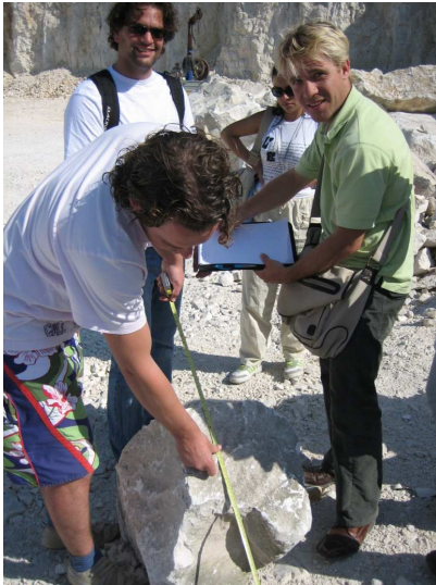
Figure 15 Determination of elongation and blockiness
