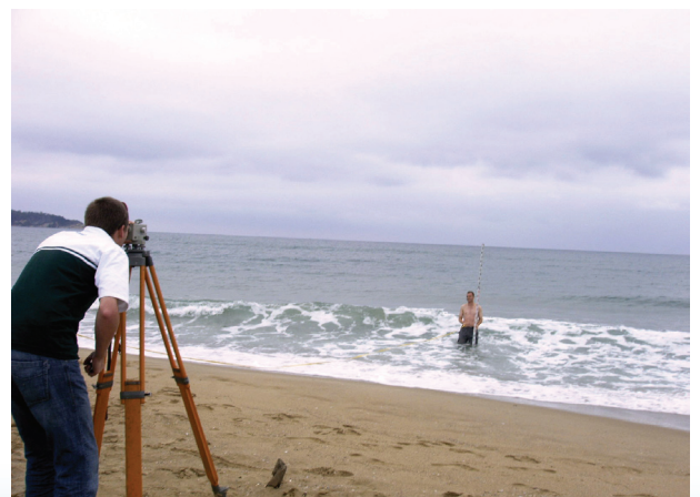
figure 2.9 Measuring the beach by using a leveling instrument
