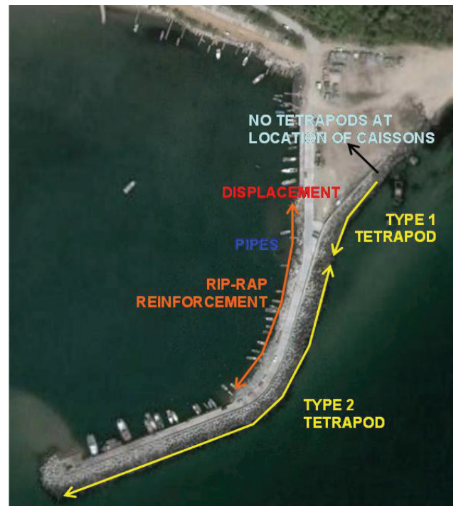
figure 7.7 Tetrapod breakwater
