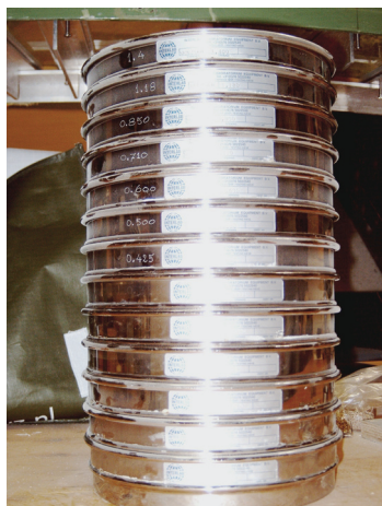
figure 5.2 Stack of sieves
