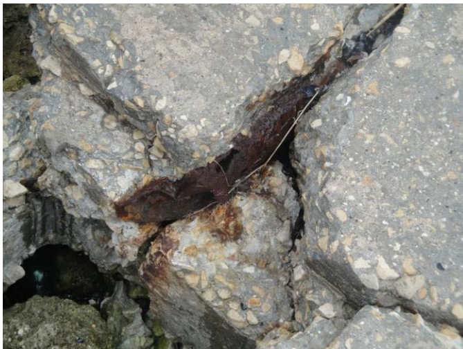
Figure 31: The remaining of an iron pipe.
