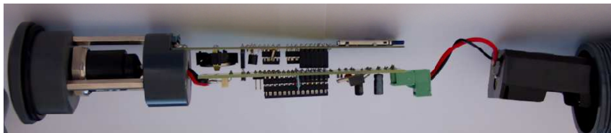
Figure 5.2 The inside of the pressure meter
