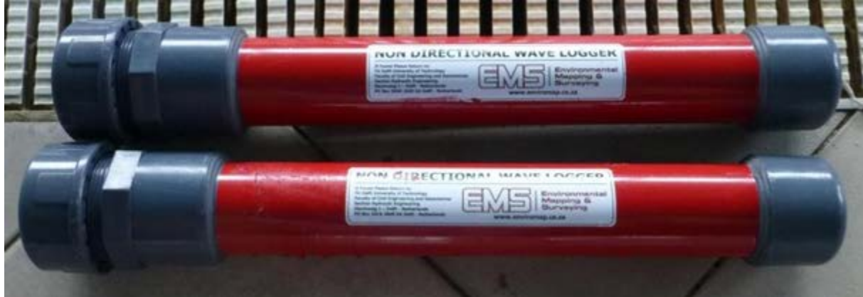
Figure 1: Environment Mapping & Surveying (EMS) non-directional wave loggers
