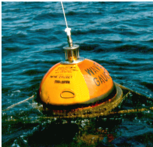
Figure 3.1 An example of a wave buoy
