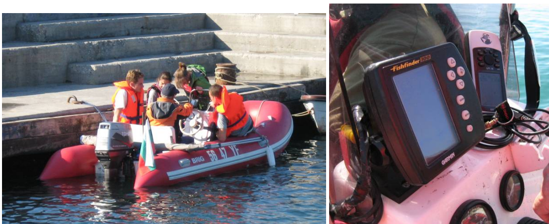
Figure 4-7: The measuring equipment. Left: rubber boat. Right: Fishfinder echosounder and Garmin GPS device
