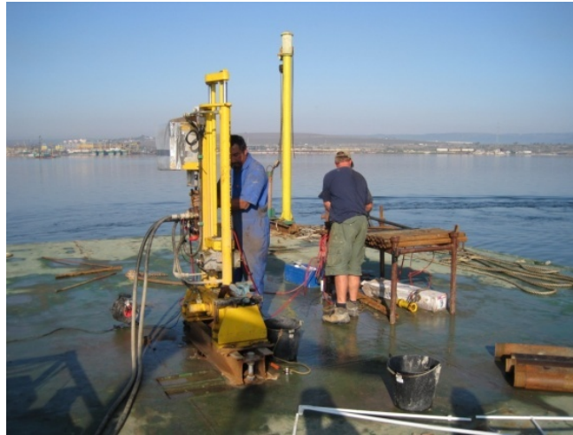
Figure 2-25: Cone penetration Test at pontoon
