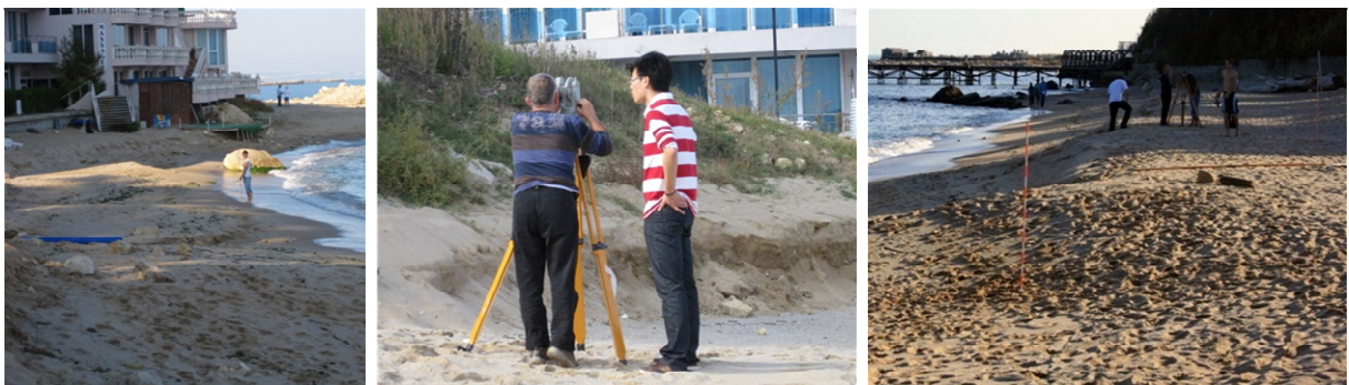
Figure 4-18: profile 75 N, complete beach disappeared, waterline is retreating
