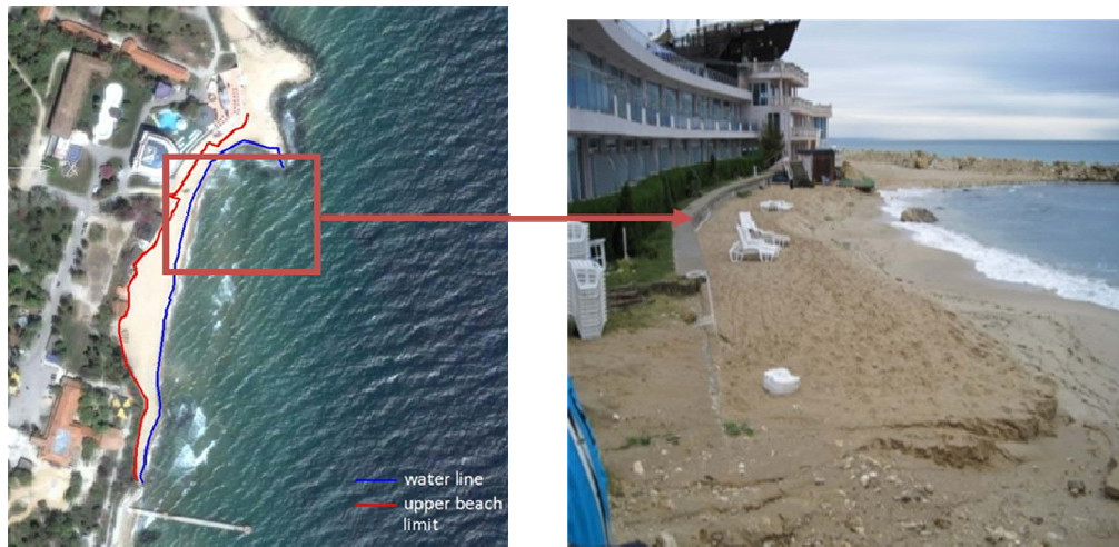
Figure 4-9: Sirius beach, retreating waterline and eroding beach
