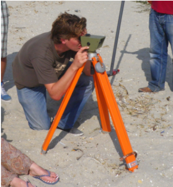
Figure 2-11 Use of the theodolite
