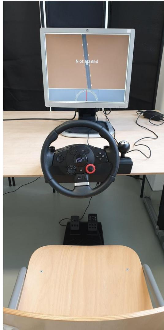
Figure 1: The used experimental setup as seen from the view of one of the participants.
