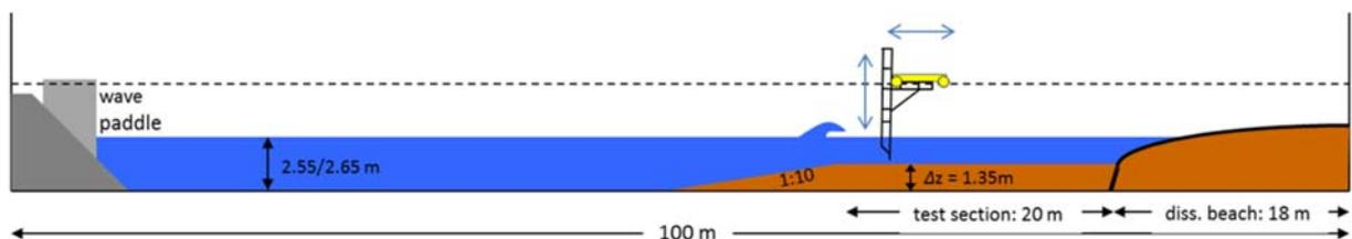
Figure 1. Mobile frame instrumentation (upper) and experimental set-up (lower).
