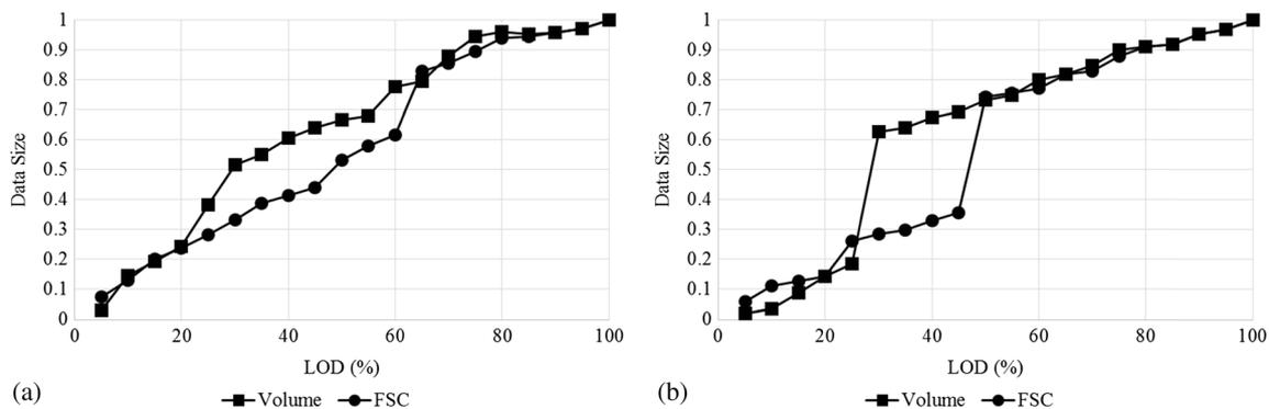
**Fig. 7** Decrease in data size during simplification. **a** Hydrophore. **b** Horizontal pump model
