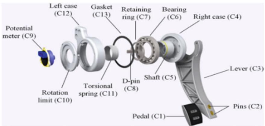
**Fig. 71.6** Exploded view of throttle pedal [8]
