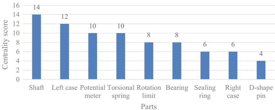
**Fig. 71.8** Centrality score of the throttle pedal
