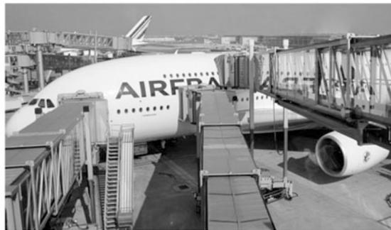
Passenger bridges connected to an Airbus A380\*\*
