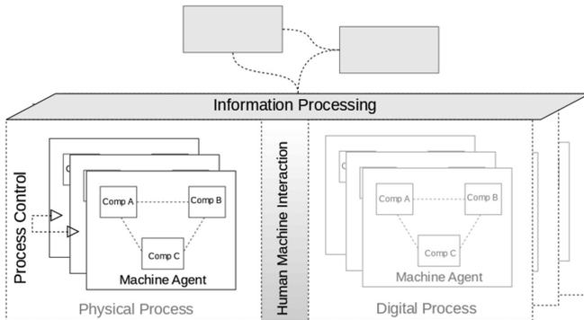
Fig. 1. General model of a digitalized manufacturing system.
