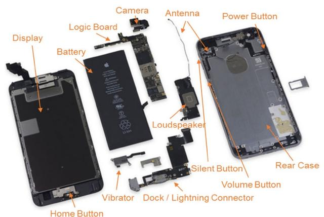
Fig. 4 Example of smartphone assemblies (iFixit 2015)
