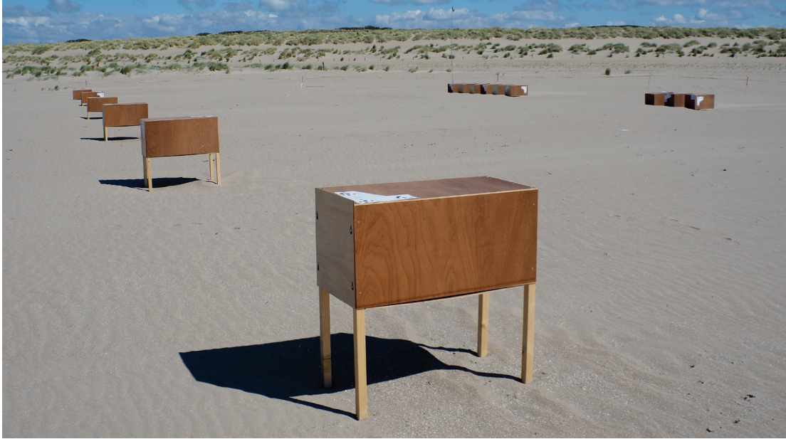
Figure 9: Photo of experiment H, with the scale models with varying pole height on the left, and two of the set-ups with varying group size in the background on the right.
