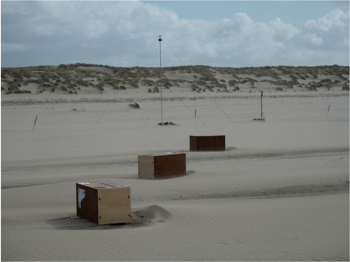
Figure 7: Photo of three of the scale models of experiment F, with the timelapse camera, WindSonic wind sensor and Wenglor particle counters in the background.
