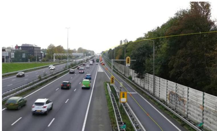
Merging the data of these lines over the frames results in pictures of moving vehicles and some stationary objects that are located on the yellow line, such as the yellow traffic light, the white stop line and the grey traffic light pole.
