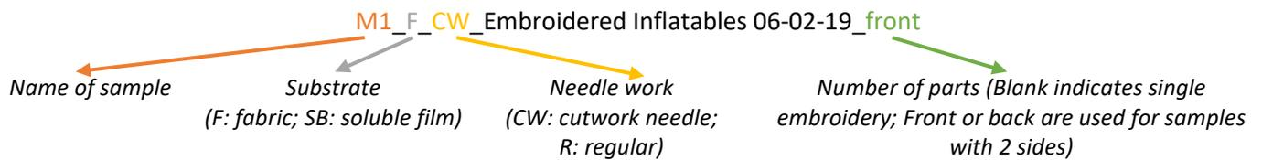
**Warning:** for CW samples, the machine needs to be set to **cutwork needle mode on** and the **4 cutwork needles need to be installed**. If the machine refuses to read file, check settings.
