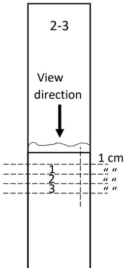
Cross-sections were later on analyzed in a Keyence digital microscope with (mostly) 400x for zoomed micrographs (in labelling supplemented by L (left), M (middle) or R (right) designating more or less the position within the micrograph) and 200x for stitched overview micrographs.
