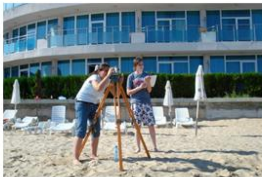
FIGURE 2-8 - PROCEDURE OF MEASURING A VERTICAL POSITION WITH A THEODOLITE
