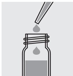
Pipette 5.0 ml of sample into a reaction cell and mix.
