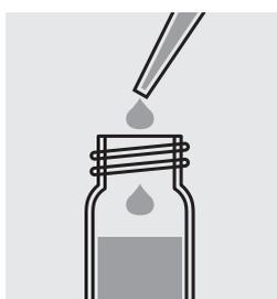
Pipette 0.50 ml of sample into a reaction cell, close the cell with the screw cap and mix.
