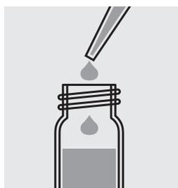
Carefully pipette 2.0 ml of sample into the cell, close with screw cap and mix vigorously. **Caution, cell becomes very hot!**
