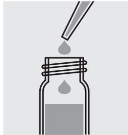
Add 0.50 ml of sample, close cell with screw cap and mix.
