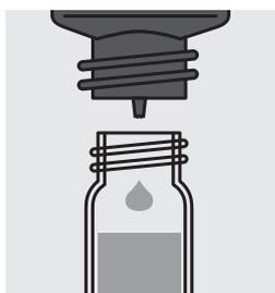
Add 5 drops of PO<sub>4</sub>-1K, close the cell with the screw cap and mix.
