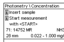
The meter is ready for the photometric measurement (step 2). The measuring range is shown on the display.
