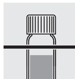
Place the cell in the cell rack again and let it cool down to room temperature (=prepared sample).
