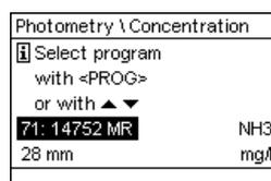
Switch to the *Photometry* measuring mode and select program no. 71.
