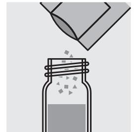
Add the contents of a **VARIO Sodium Periodate F10** powder pack and close the cell with the screw cap.
