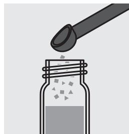
Add 1 level blue microspoon of **K-2K** and close the cell with the screw cap.
