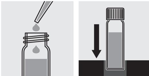
Pipette 5.0 ml of sample into a reaction cell, close the cell with the screw cap and mix.
