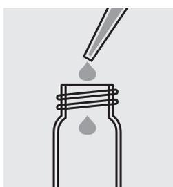
Pipette 2.0 ml of sample into a reaction cell, close the cell with the screw cap and mix.
