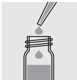
Carefully add 1.5 ml of sample with a pipette, close the cell with the screw cap and mix. **Caution, cell becomes very hot!**
