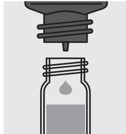
Add 5 drops of **Cu-1K**, close cell with screw cap and mix.
