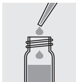
Add 8.0 ml sample with a pipette, close the cell with the screw cap and mix.
