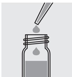
Using a pipette, add 0.50 ml of **Zn-2K** into a reaction cell and close the cell with the screw cap.
