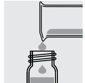
Fill an empty cell with the prepared sample and close it with the screw cap.
