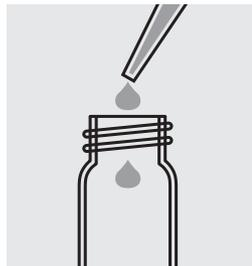
Pipette 1.0 ml of sample into the empty cell.
