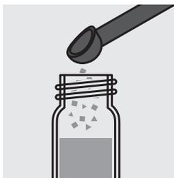
Add 1 level blue microspoon of **NO<sub>3</sub>-1K** into a reaction cell and close the cell with the screw cap.
