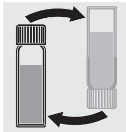
Mix the contents by carefully swaying the cell (10 x). Undissolved powder has no adverse effect on measurement.
