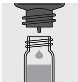
Add 5 drops of **Zn-1K** into a reaction cell, close the cell with the screw cap and mix.
