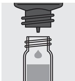
Add 6 drops of **N-2K**, close cell with screw cap and mix.
