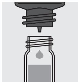
Add 4 drops of **Mn-3**, close the cell with the screw cap and mix.
