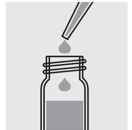
Add 0.50 ml **Al-3** with a pipette, close the cell with the screw cap and mix.
