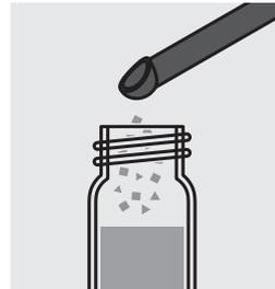
Add 1 level green microspoon of **Cd-2K** and close the cell with the screw cap.
