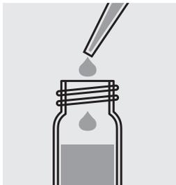
Pipette 0.50 ml of sample into a reaction cell and mix.
