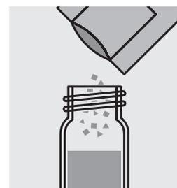
Add the contents of a **VARIO Hexamine F20** powder pack and close the cell with the screw cap.
