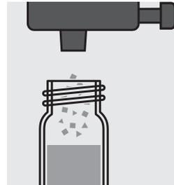
Add one dose of **P-1K** with the green measurer and close the cell with the screw cap.
