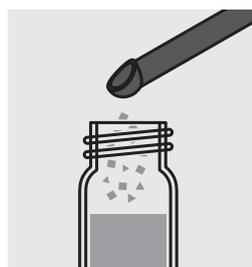
Add 1 level green microspoon of SO<sub>4</sub>-1K and close the cell with the screw cap.
