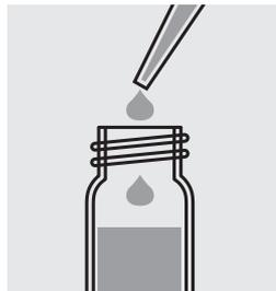
**Carefully** pipette 3.0 ml of sample into the cell, close with screw cap and mix vigorously.
