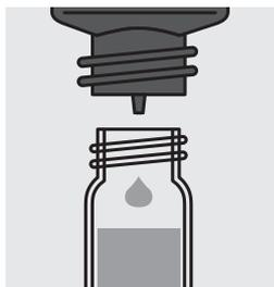
Add 5 drops of **P-2K**, close cell with screw cap and mix.
