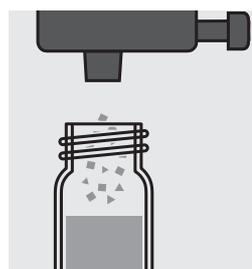
Add 1 dose of **NH<sub>4</sub>-1K** with the blue measurer and close the cell with the screw cap.
