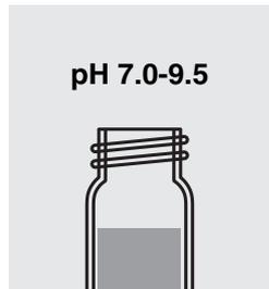
Check the pH value. Desired range: pH 7.0-9.5. Correct with diluted sodium hydroxide solution or sulfuric acid as necessary.
