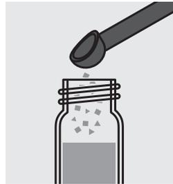
Add 1 level black measuring spoon no. 8 of **Nitrit-101** and close the cell with the screw cap.
