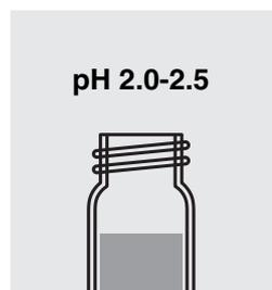
Check the pH value. Desired range: pH 2.0-2.5. Correct with diluted sodium hydroxide solution or sulfuric acid as necessary.
