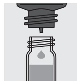
Add 4 drops of **PO<sub>4</sub>-4**, close the cell with the screw cap and mix.
