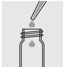
Pipette 10 ml sample into the empty cell.
