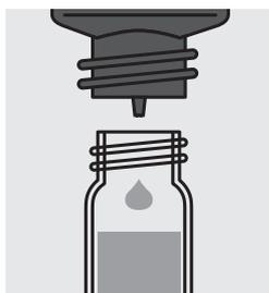
Add 4 drops of **PO<sub>4</sub>-4**, close the cell with the screw cap and mix.
