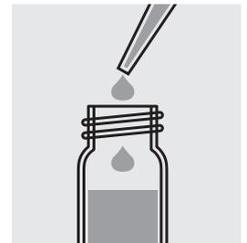
Add 5.0 ml sample with a pipette, close the cell with the screw cap and mix.
