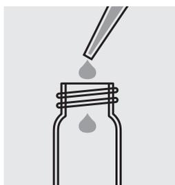
Pipette 0.10 ml of sample into the empty cell.
