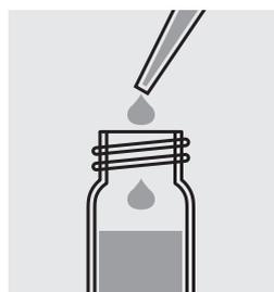
Carefully add 2.0 ml of the **prepared sample** with a pipette, close the cell with the screw cap and mix.
