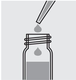
Pipette 0.50 ml **Na-1K** into a reaction cell and mix.
