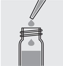
Pipette 4.0 ml of sample into a reaction cell and close the cell with the screw cap.
