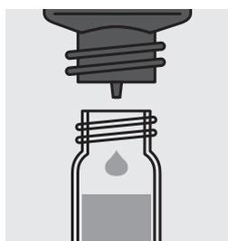
Add 8 drops of **NH<sub>4</sub>-3**, close the cell with the screw cap and mix.
