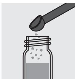
Add 1 level blue microspoon of **Fe-1K** and close the cell with the screw cap.
