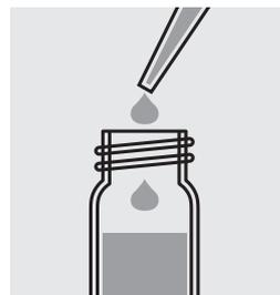
Using a pipette, add 6.0 ml **Au-4A** and close the tube.
