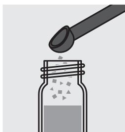
Add 2 level blue microspoons of **NO<sub>2</sub>-1** and close the cell with the screw cap.
