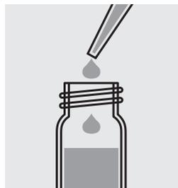
Add 1.0 ml **H-1K** with a pipette, close the cell with the screw cap and mix.
