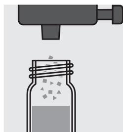
Add 1 dose of **P-3K** with the blue measurer and close the cell with the screw cap.
