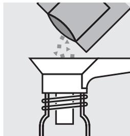
Add the contents of a **VARIO TN Reagent B** powder pack, close the cell with the screw cap and mix for at least 15 s.
