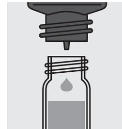
Add 5 drops of **Cu-2**, close cell with screw cap and mix.
