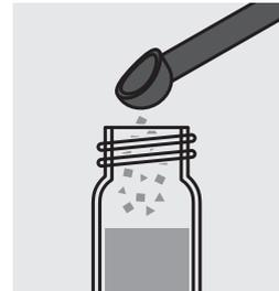
Add one level blue microspoon of ClO<sub>2</sub>-2 and close the cell with the screw cap.
