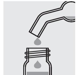
Fill the solution from the absorption tube into an empty cell.
