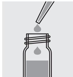
Pipette 2.0 ml of prepared sample into a **TN Acid LR/HR (Reagent C)** reaction cell and close the cell with the screw cap.
