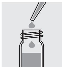
Add 1.0 ml sample with a pipette, close the cell with the screw cap and mix.
