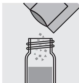
Add the contents of a **VARIO Ferro F10** powder pack and close the cell with the screw cap.
