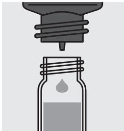
Add 4 drops of NH<sub>4</sub>-3, close the cell with the screw cap and mix.
