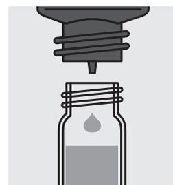
Add 5 drops of **Zn-3K**, close cell with screw cap and mix.
