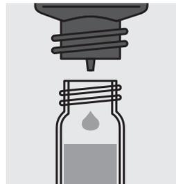
Add 6 drops of **Cr-3K** into a reaction cell and close with screw cap.
