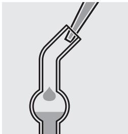
Pipette 5.0 ml **As-5** into the AS absorption tube (WTW article no. 252 066).
