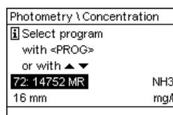
Switch to the *Photometry* measuring mode and select program no. 72.
