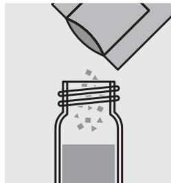
Add the contents of a **VARIO MANGANESE Citrate Buffer F10** powder pack and close the cell with the screw cap.
