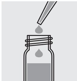
Add 0.20 ml **AC-2** with a pipette, close the cell with the screw cap and mix.
