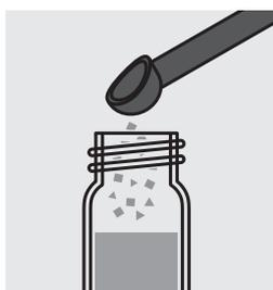
Add 1 level blue microspoon of **CN-3K** and close the cell with the screw cap.
