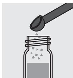
Add 2 level blue microspones of **PO<sub>4</sub>-2** and close the cell with the screw cap.
