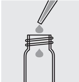
Pipette 5.0 ml of sample into a reaction cell.
