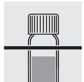
Remove the reaction cell from the thermoreactor and let it cool down to room temperature in a cell rack.
