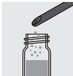
Add two level gray microspoons of NO<sub>3</sub>-3 and close the cell with the screw cap.
