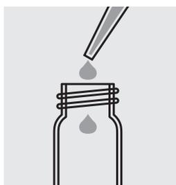
Pipette 5.0 ml of sample into the empty cell.
