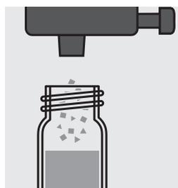
Add 1 dose of **P-1K** with the green measurer and close the cell with the screw cap.
