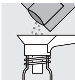
Add the contents of a **VARIO Phos 3 F10** powder pack and close the cell with the screw cap.
