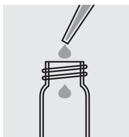
Pipette 4.0 ml of sample into the empty cell.
