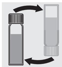
Mix the contents by carefully swaying the cell (10 x). A small amount of solids may remain undissolved.
