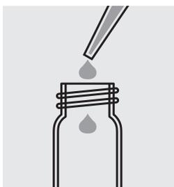
Pipette 5.0 ml of **AC-1** into the cell.
