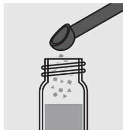
Add one level blue microspoon of O<sub>3</sub>-2 and close the cell with the screw cap.
