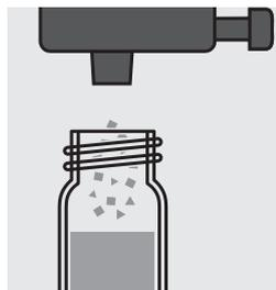
Add one dose of **P-3K** with the blue measurer and close the cell with the screw cap.
