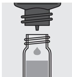
Add 5 drops of **Zn-2K**, close cell with screw cap and mix.
