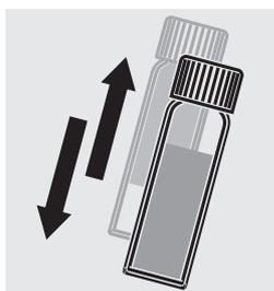
To dissolve solids, shake the cell for approx. 10 to 15 seconds. A small amount of solids may remain undissolved.
