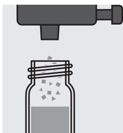
Add 1 dose of **PO<sub>4</sub>-2** with the green measurer and close the cell with the screw cap.
