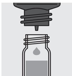
Add 3 drops of **Fe-AN**, close the cell with the screw cap and mix.
