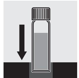
Insert the cell in the photometer cell shaft within one minute and start measurement.
