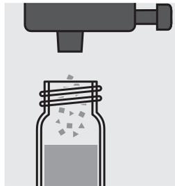
Add 1 dose of NH<sub>4</sub>-2 with the blue measurer and close the cell with the screw cap.
