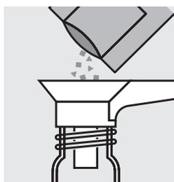
**Add the contents of a VARIO Potassium Persulfate F10** powder pack and close the cell with the screw cap.
