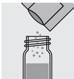
Add the contents of a **VARIO Nitrate Chromotropic** powder pack and close the cell with the screw cap.
