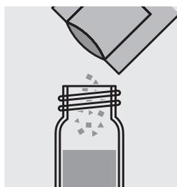
Add the contents of a **VARIO Aluminium ECR F20** powder pack and close the cell with the screw cap.
