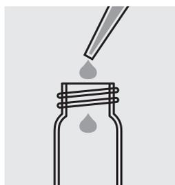
Pipette 0.50 ml of **Pb-1** into the empty cell.
