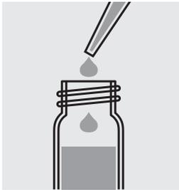
Pipette 5.0 ml of sample into a reaction cell and close the cell with the screw cap.
