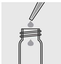
Pipette 10.0 ml of sample into an empty cell.
