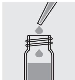
Add 1.0 ml **Mg-1K** with a pipette, close the cell with the screw cap and mix.
