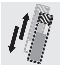
Shake the cell for 10 to 15 seconds. Undissolved powder has no adverse effect on measurement.
