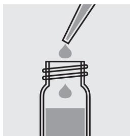
With a pipette add 2.0 ml of 1.54 N sodium hydroxide solution, close the cell with the screw cap and mix the contents by carefully swaying the cell.
