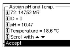
When the prompt *Assign pH und temp.* appears, select and accept the stored values from the pH and temperature measurement.
