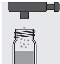
Add 1 dose of PO<sub>4</sub>-2K with the blue measurer and close the cell with the screw cap.
