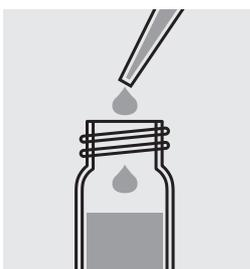
Add 0.50 ml of sample with a pipette, close the cell with the screw cap and mix.
