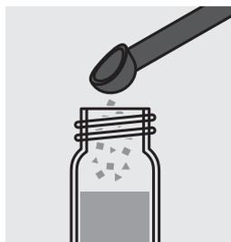
Add 1 level blue microspoon of **N-3K** into a reaction cell and close the cell with the screw cap.
