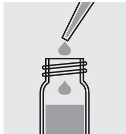
Add 1.0 ml of sample with a pipette, close the cell with the screw cap and mix.
