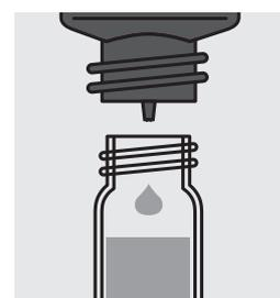
Add 6 drops of **K-1K**, close cell with screw cap and mix.
