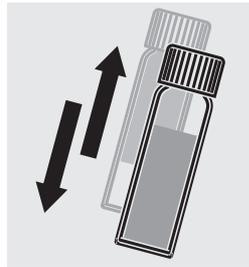
To dissolve solids, shake the cell vigorously for approx. 30 seconds.
