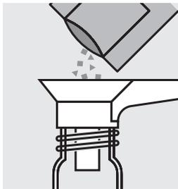
Add the contents of a **VARIO TN Persulfate Rgt.** powder pack into a **TN Hydroxide HR** digestion cell.
