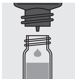
Add 15 drops of **Vario Molybdate 3 Reagent Solution** and close the cell with the screw cap.
