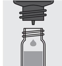
Add 2 drops of Cl<sub>2</sub>-2, close the cell with the screw cap and mix.
