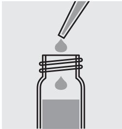
Pipette 2.0 ml of sample into a reaction cell.
