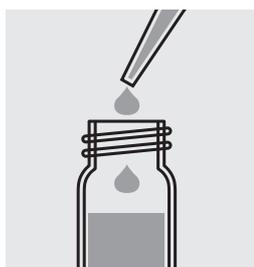
Pipette 5.0 ml of sample into a reaction cell and dissolve solids.
