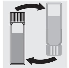
Mix the contents by carefully swaying the cell (10 x).
