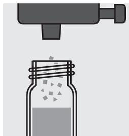
Add 1 dose of **PO<sub>4</sub>-3** with the blue measurer and close the cell with the screw cap.
