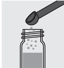
Add 2 level blue microspoons of NH<sub>4</sub>-2 and close the cell with the screw cap.
