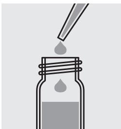
Add 0.50 ml of sample with a pipette and mix.
