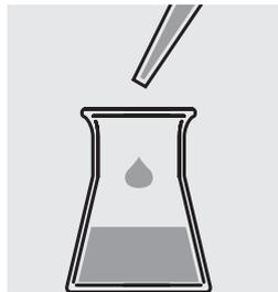
Using a pipette, add 1.0 ml **As-6** to the solution in the Erlenmeyer flask and mix.
