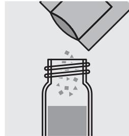
Add the contents of a **MolyVer 2 Reagenz** powder pack and close the cell with the screw cap.
