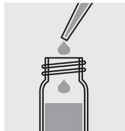
Pipette 1.0 ml of sample into a reaction cell and mix.
