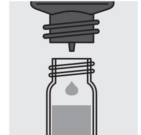
Add 3 drops of **Mn-2K**, close cell with screw cap and mix.
