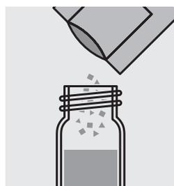
Add the contents of a **VARIO AMMONIA Cyanurate F5** powder pack and close the cell with the screw cap.
