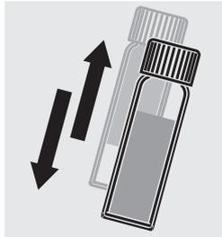
Shake the cell vigorously to dissolve solids. A small amount of solids may remain undissolved.
