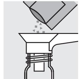
Add the contents of a **VARIO TN Reagent A** powder pack, close the cell with the screw cap and mix for at least 15 s.
