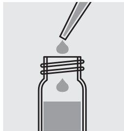
With a pipette add 2.0 ml of sample, close the cell with the screw cap and mix vigorously for at least 30 s. A small amount of solids may remain undissolved.
