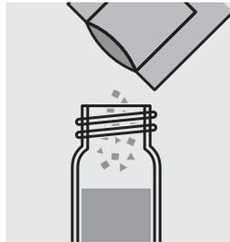
Add the contents of one **VARIO Chlorine Total DPD PP** powder pack and close the cell with the screw cap.
