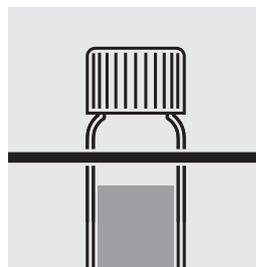
Place the cell in the cell rack again and let it cool down to room temperature.
