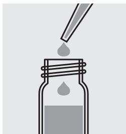
With a pipette add 1.5 ml of prepared sample very slowly, close with screw cap and mix vigorously. **Caution, cell becomes very hot!**
