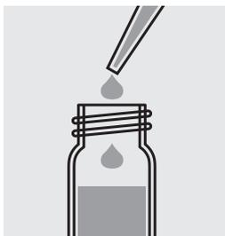
Pipette 2.0 ml of the sample into a test tube with screw cap.
