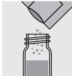
Add the contents of a **VARIO Cu1 F10** powder pack and close the cell with the screw cap.
