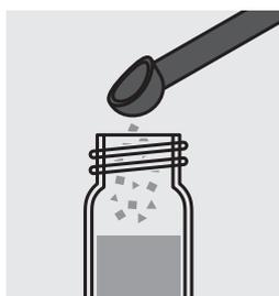
Add 1 level blue microspoon of Cl<sub>2</sub>-1 and close the cell with the screw cap.
