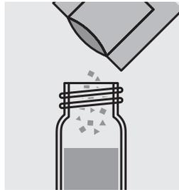
Add the contents of a **VARIO SULPHA 4 F10** powder pack and close the cell with the screw cap.
