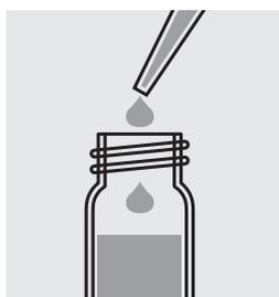
**Carefully** pipette 2.0 ml of sample into the cell, close with screw cap and mix vigorously.
