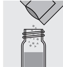
Add the contents of a **VARIO AMMONIA Cyanurate F10** powder pack and close the cell with the screw cap.
