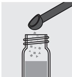
Add 1 level blue microspoon of NH<sub>4</sub>-2 and close the cell with the screw cap.
