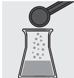
Add two level red measuring spoons of granulated zinc and **immediately** attach the filled absorption tube on the Erlenmeyer flask.
