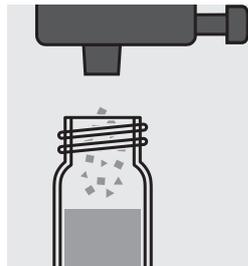
Add 1 dose of **PO<sub>4</sub>-2** with the green measurer and close the cell with the screw cap.
