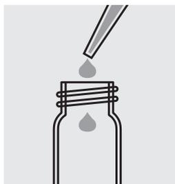
Pipette 8.0 ml of deionized water into the empty cell.
