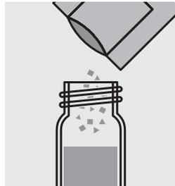
Add the contents of a **VARIO Chlorine FREE-DPD/F10** powder pack and close the cell with the screw cap.
