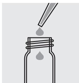
Pipette 10.0 ml sample into the empty cell.
