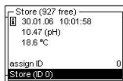
Store measured values with <STO>. If necessary, assign an ID for easier retrieving.
