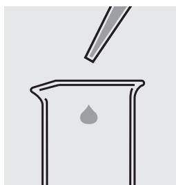
Pipette 10.0 ml of sample into an empty beaker.
