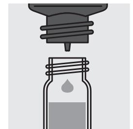
Add 3 drops of **Mg-2K**, close cell with screw cap and mix.
