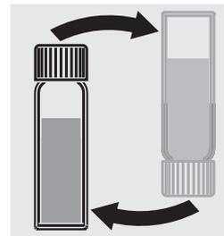
Mix the contents by carefully swaying the cell (10 x).
