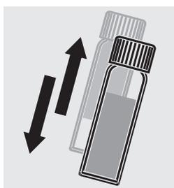
To dissolve solids, shake the cell **vigorously for 5 seconds**.
