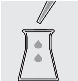
Fill 350 ml of the sample into an Erlenmeyer flask with ground joint.
