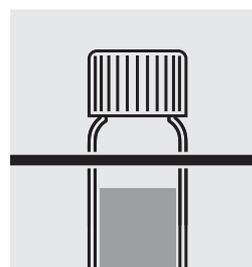
Remove the reaction cell from the thermoreactor and let it cool down to room temperature in a cell rack.
