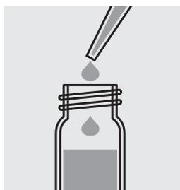
Add 1.00 ml **Si-3** with a pipette, close the cell with the screw cap and mix.
