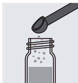
Add 1 level blue microspoon of PO<sub>4</sub>-2 and close the cell with the screw cap.
