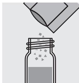
Add the contents of a **VARIO LR Silica Amino Acid F F10** powder pack and close the cell with the screw cap.
