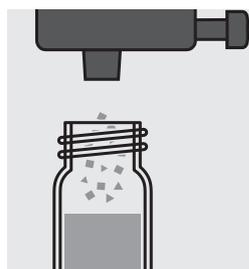
Add 1 dose of **F1-K** with the blue measurer and close the cell with the screw cap.
