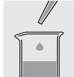
Add 15.0 ml deionized water with a pipette and mix.
