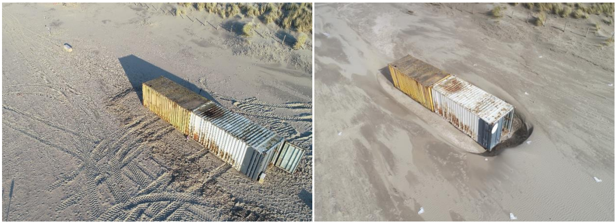
Figure 7: Experiment B. Left: the small and full-scale model upon placement Day0, 06-02-2020). Right, the full-scale model after approximately 5 weeks (11-03-2020, referred to as 'Day4', because it is the fourth measurement day).
