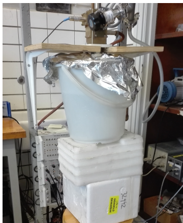
(a) Cooling down the set-up. The bucket is filled with ice water.
