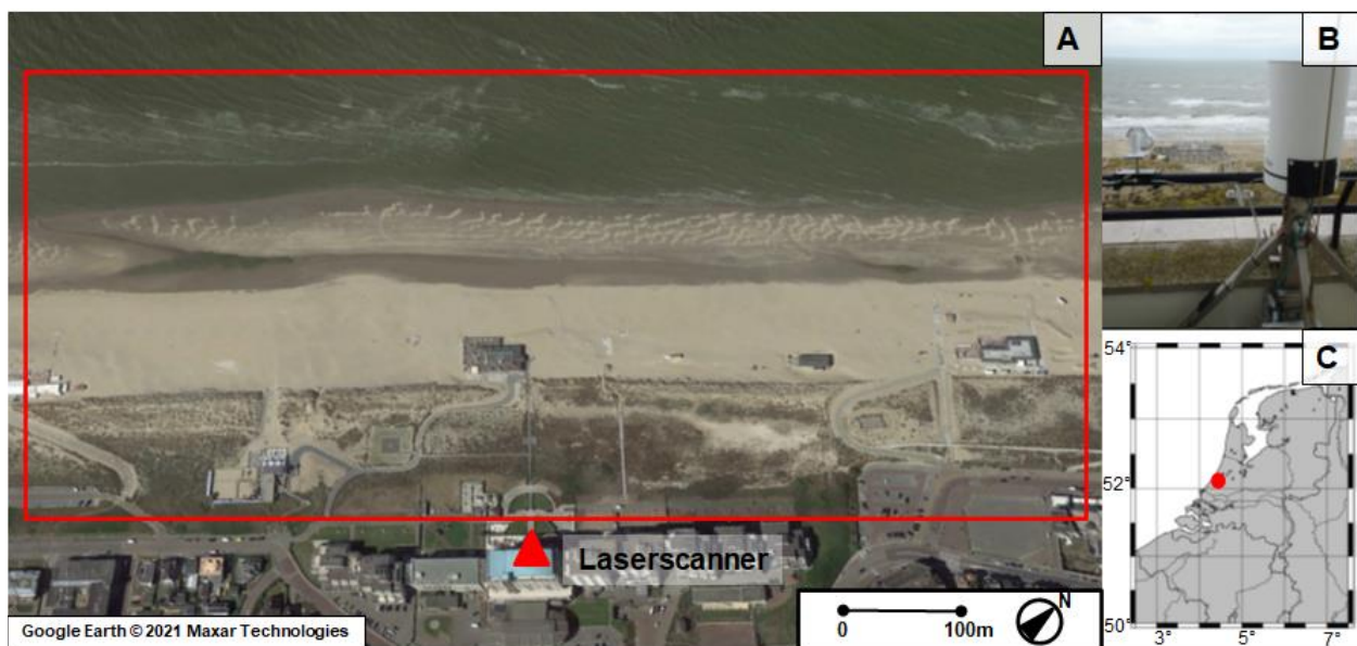
Figure 1: (A) Aerial photo of the beach-dune system in Noordwijk and the scan area within the red rectangle. (B) The laser scanner positioned on a hotel facing the beach (indicated by a red triangle in A). (C) The location of Noordwijk (52.24°N, 4.42°E) in The Netherlands.
