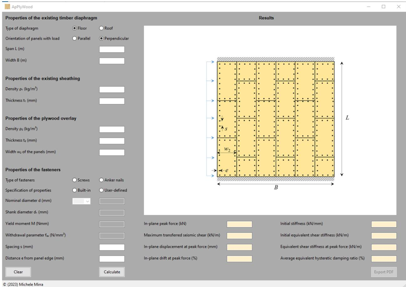
Next, the span  $L$  has to be specified (in m; this is the dimension orthogonal to the in-plane distributed load), along with the width  $B$  (in m; this is the dimension orthogonal to the in-plane distributed load).
