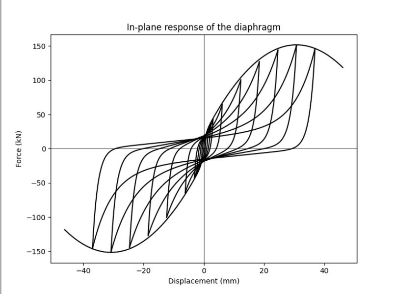
The graph displays the in-plane response of the diaphragm, plotting Force (kN) on the y-axis (ranging from -150 to 150) against Displacement (mm) on the x-axis (ranging from -40 to 40). It shows several hysteretic cycles, indicating the load-unload-reload behavior of the diaphragm under seismic loading.
