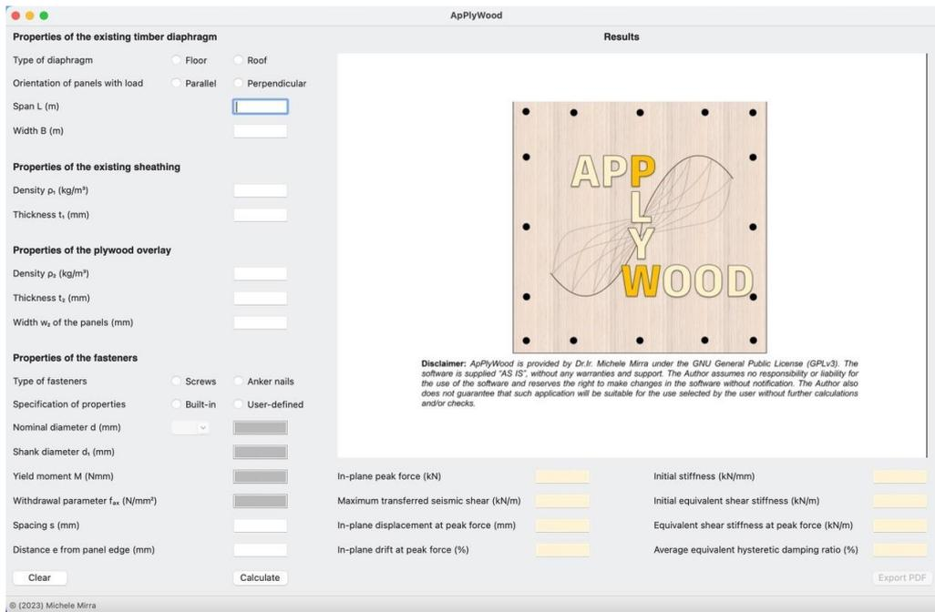
The user needs to first specify the type of diaphragm (floor or roof; in the latter case, the span to be specified is the inclined length of one in-plane loaded pitch), the panel orientation with respect to the load (parallel or perpendicular), and the main dimensions  $L$  and  $B$ . During the selection, a schematic picture of the diaphragm appears, to help the user specify all required parameters.
